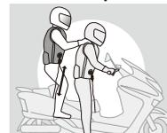
A wire fixed to the rear seat. Standing on the rear step in a half crouching position and the wire is at full length
