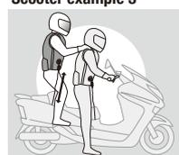
A wire fixed to the rear seat. Standing on the rear step in a half-crouching position and the wire is at full length
