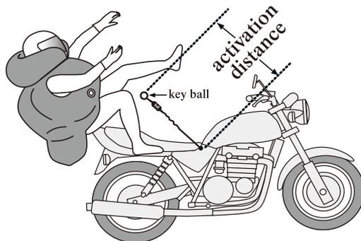
The jacket with the Hit-Air (Shock-buffering Protection System) is to be worn as an outerwear when riding a motorcycle.
