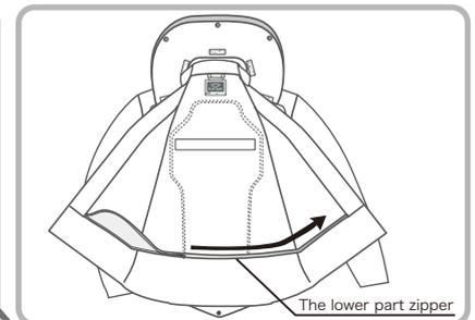
Airbag systems are attached to the inside of the vest/jacket with zippers in 3 places, the back cushion(A) and the body cushion(B,C).
