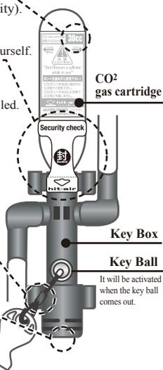
**①** The size (capacity) of the cartridge varies from model to model. Make sure that the size (capacity) shown on the seal attached to the CO<sup>2</sup> cartridge and that shown at the back of the key box cover are the same. (\*Some model has no size label attached)
