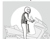
A wire fixed to the seat. Standing on the ground and the wire is at full stretch.
