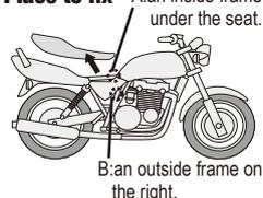
**Caution** Don't fix a coiled wire to any part where it would disturb driving the motorcycle, where it would lead to damage a part of the motorcycle, where it may come off when it is pulled and where it becomes hot (over 60°C) such as the engine or muffler.
