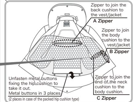
The end of the neck cushion is joined to the body cushion with the fastener(C)
