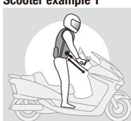
A wire fixed to the neck of the handlebar. Standing on the scooter and the wire is at full stretch
